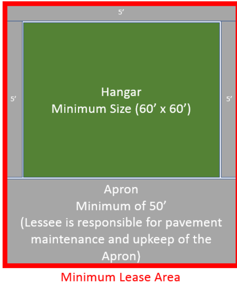
Figure A4. Private Hangar Example
